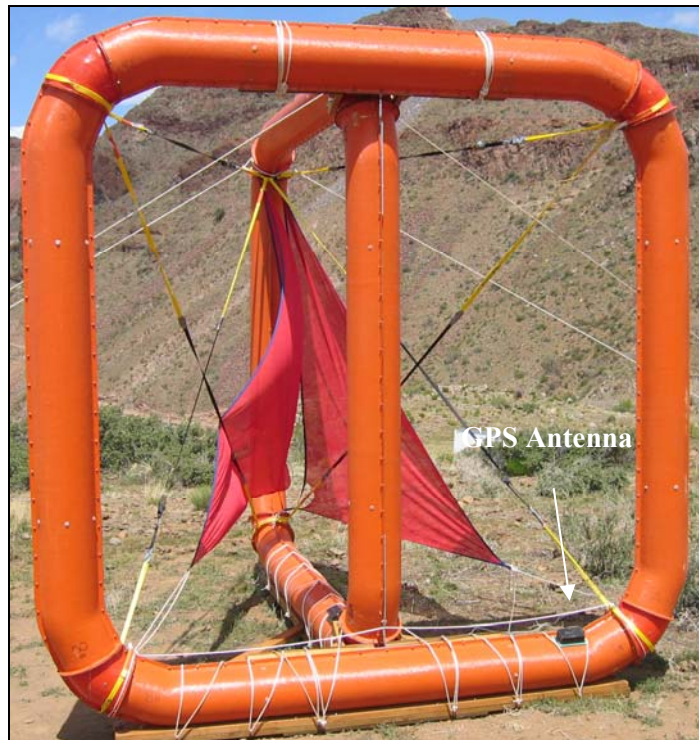
Figure 7 - ZTEM base station receiver coils.
